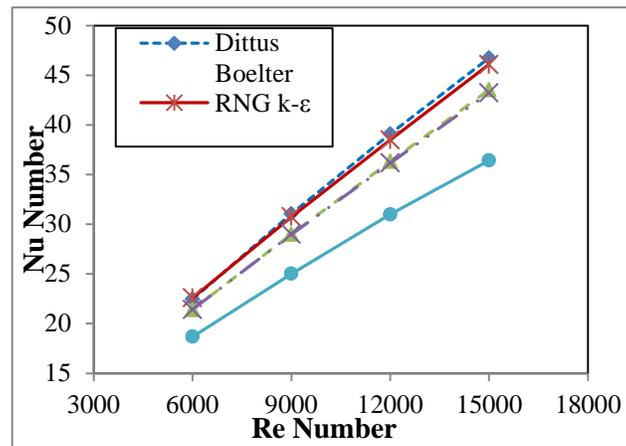
Fig.2. Comparison of different model with Dittus-Boelter empirical relation for smooth duct.
