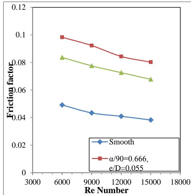
Fig. 6. Variation of Friction factor with Reynolds number for different values of relative inclination angle
