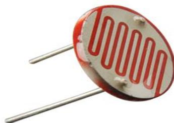
A photoresistor (or light-dependent resistor, LDR, or photo-conductive cell) is a light-controlled variable resistor. The resistance of a photoresistor decreases with increasing incident light intensity; in other words, it exhibits photoconductivity. A photoresistor can be applied in light-sensitive detector circuits, and light-activated and dark-activated switching circuits.
