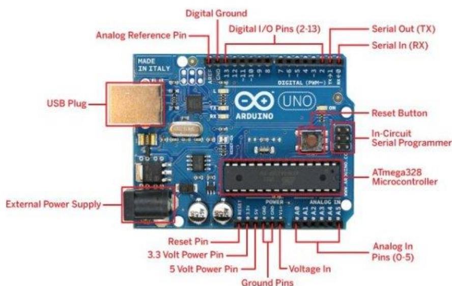
The arduino board exposes most of the microcontroller's I/O Pins for use by other circuits. The diecimila, Duemilanove, and current Uno provide 14 digital I/O Pins , six of which can produce pulse width modulated signals, six analog inputs, which can be used as a six digital I/O Pins
