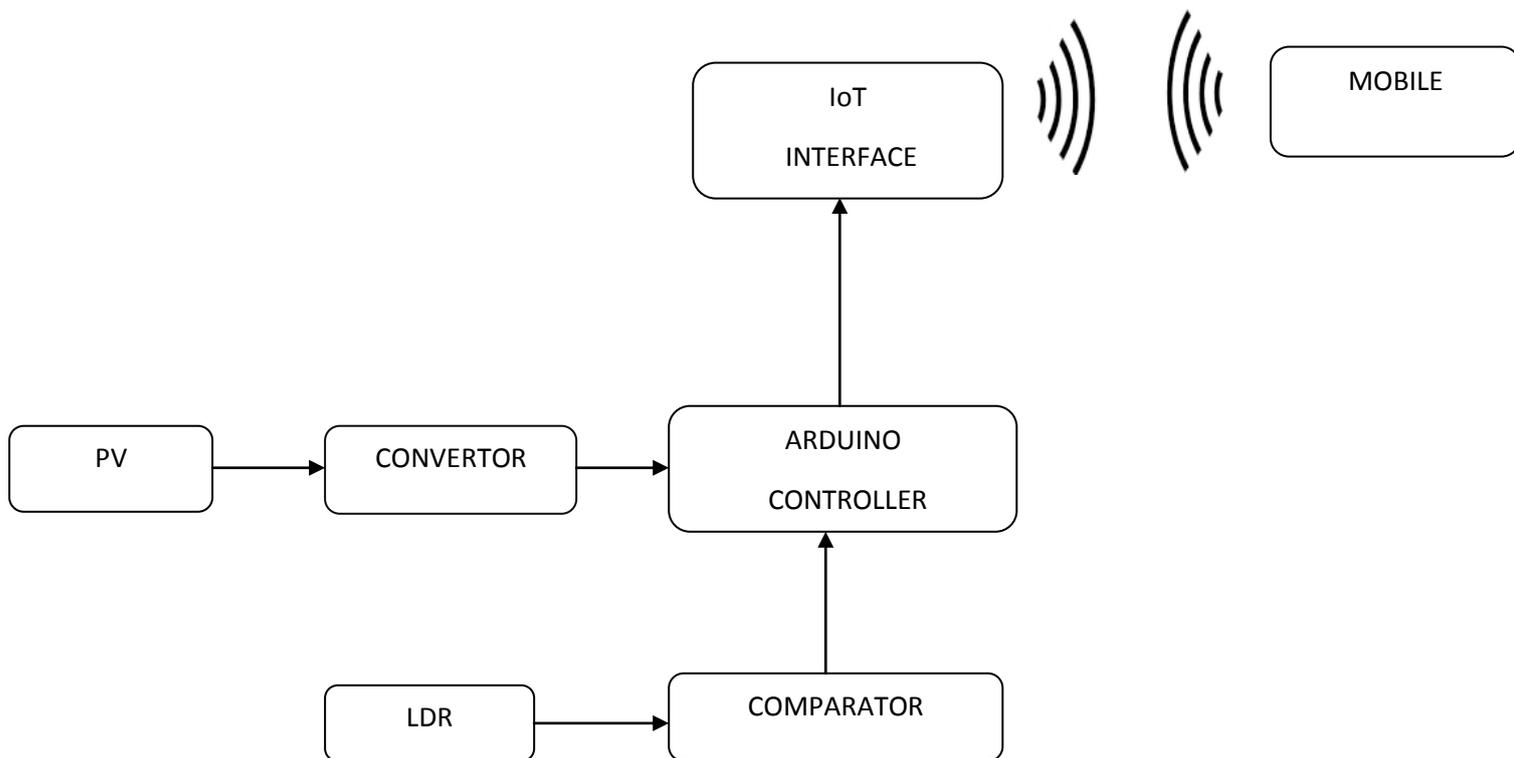
Block Diagram of fault monitoring System
