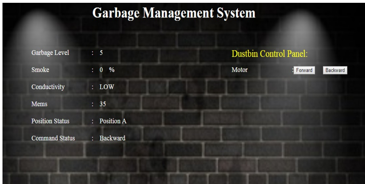
Fig 5. Webpage to monitor and control
