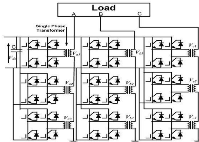
Fig. 2. The Cascaded H-Bridge MLI Structure.
