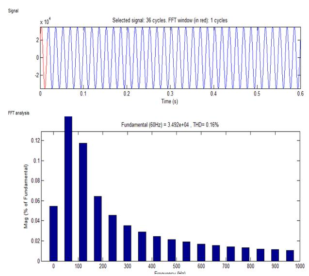
Fig.11. Proposed system harmonic distortion
