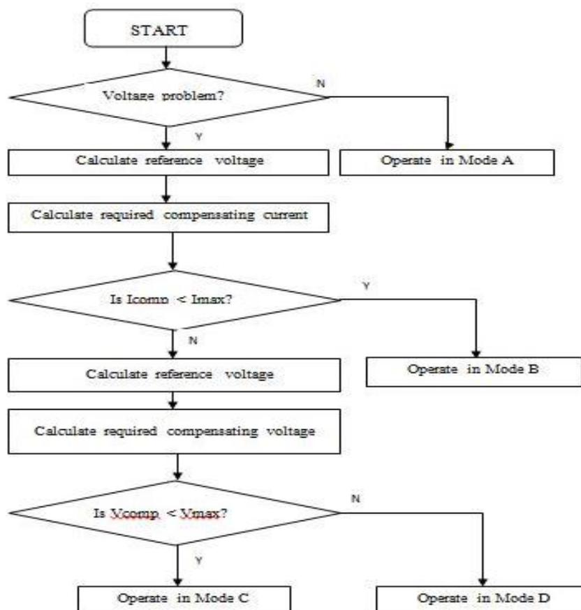
Fig.3. SSS-MLI mode transition flowchart.
