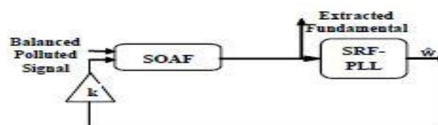
Fig. 4. Representation of conventional second order adaptive filter.
