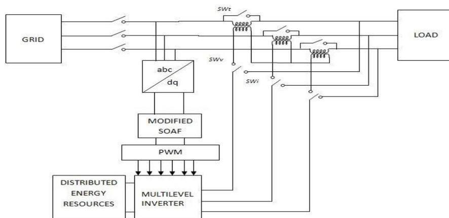
Fig. 1. The proposed system with shunt-series-switched MLI (SSS-MLI) with modified SOAF structure
