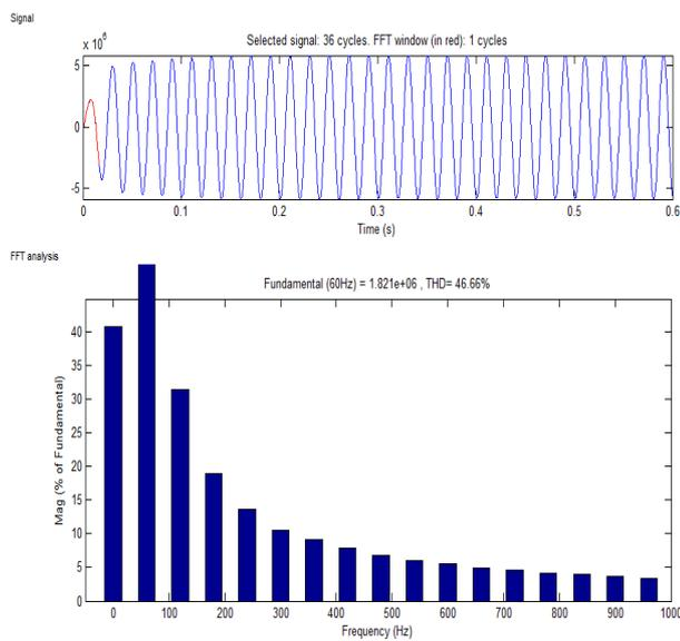
Fig. 10. Existing system harmonic distortion
