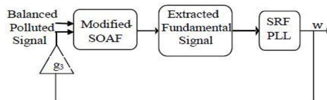
Fig. 5. Representation of modified second order adaptive filter.
