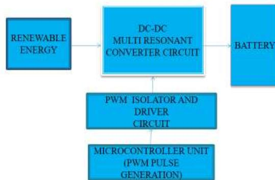
Fig no 1 Block Diagram Of Multi Resonant Converter.
