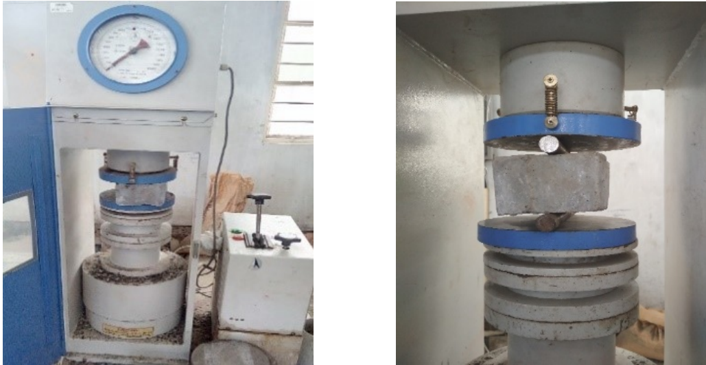
Fig. 2 Compression and Split tension test on paver blocks
