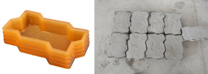
Fig. 1 Unipaver mould and Casted Unipaver blocks
