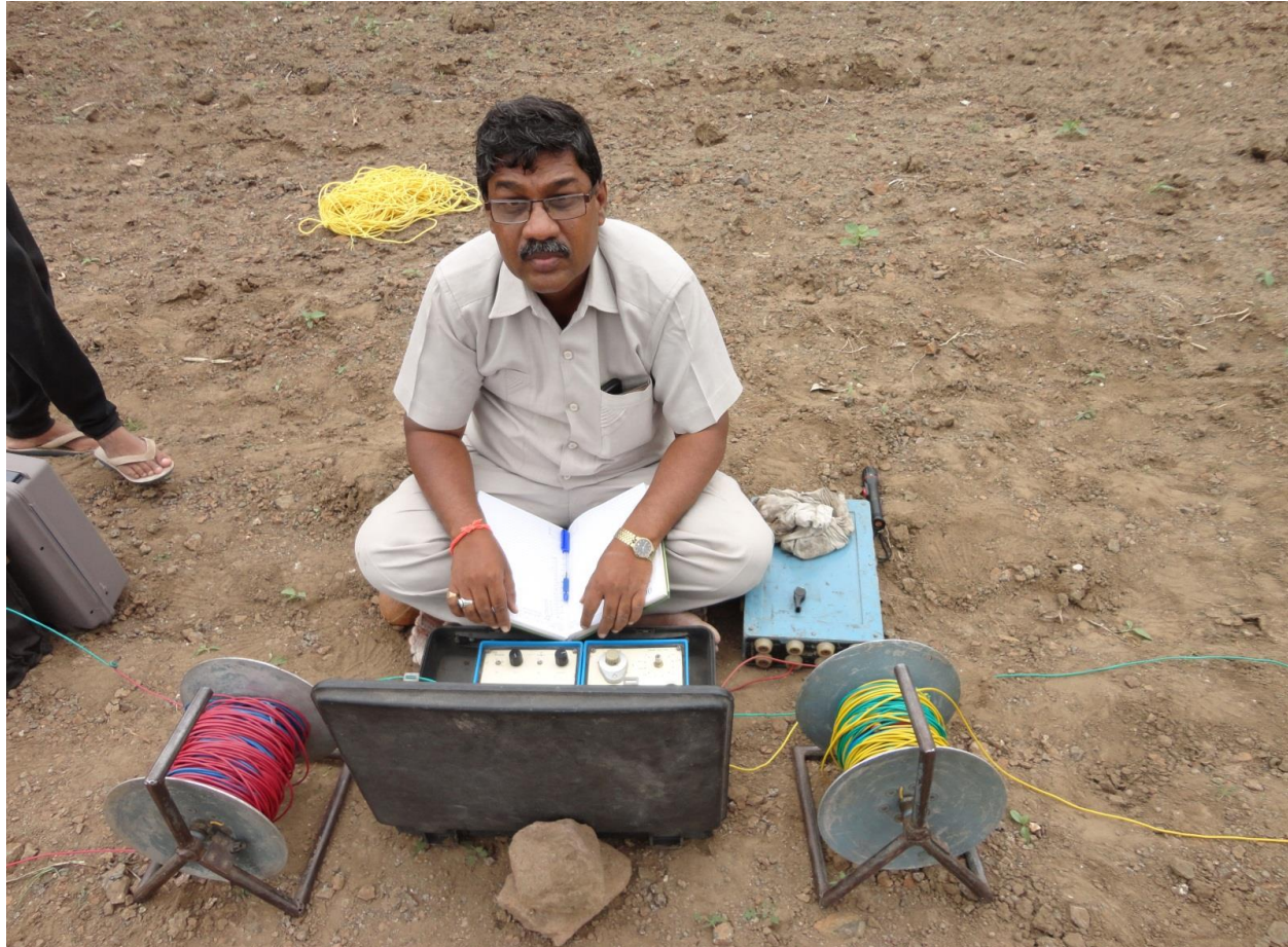
Photo 1 : Shows resistivity survey for subsurface rock identification
