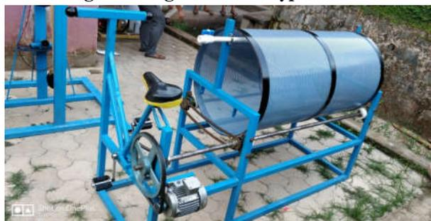
**Fig 4.2 Fabricated Barrel Type Washer**
