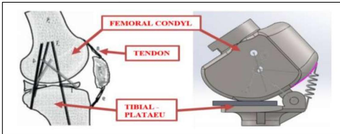
Figure 1. Structure of Human Knee Vs Prosthetic knee
