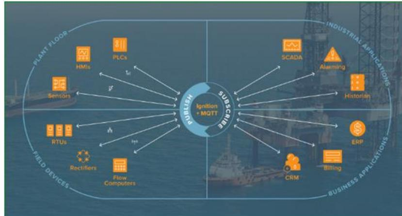
Fig.3. Architecture of MQTT protocol.
