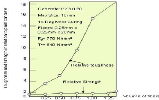
Fig.2: Effect of volume of fibers in flexure
