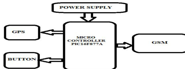
Figure 1: Block diagram for the components of tracking system
