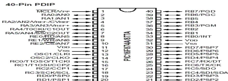
Figure 3: Pin diagram of PIC16F877A Microcontroller
