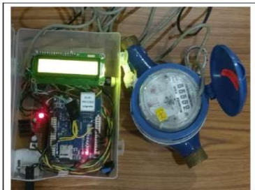
Fig. 1. Smart-meter prototype with external EIM
