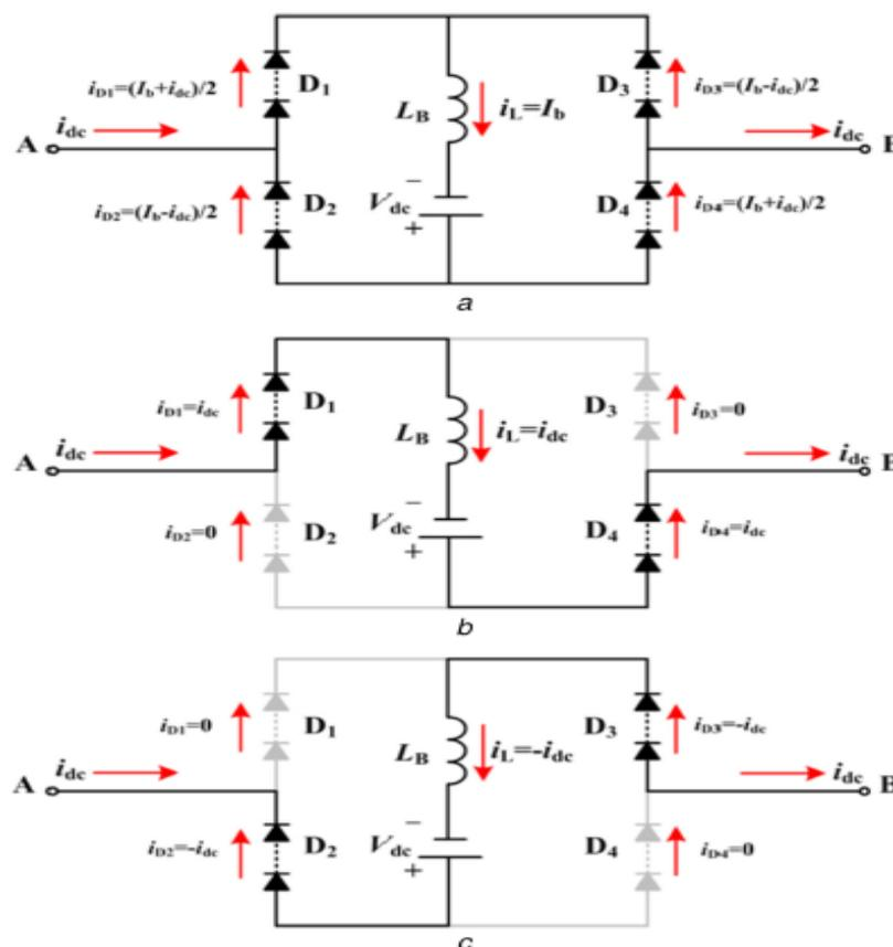
Fig 2 Working principle of the bridge-type FCL in the MMC-based dc grid(a) Current flowing path during normal operation; (b) Current flowing path during fault current limitation ( $i_{dc} > 0$ ); (c) Current flowing path during fault current limitation ( $i_{dc} < 0$ )
