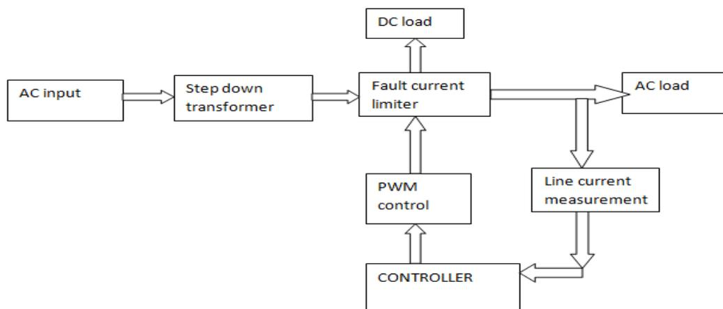
Fig.5.Proposed system for the fault current limiter using micro grid
