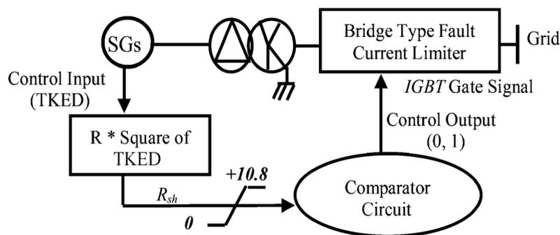
Fig.4.Static nonlinear controller connection scheme with bridge type FCL.
