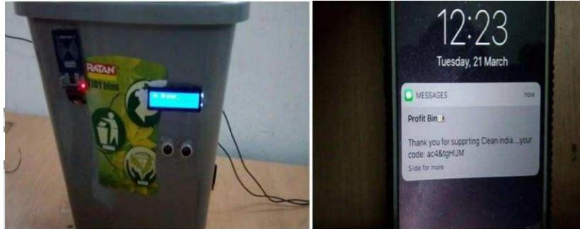
Figure 3. Dustin with mounted LCD and alert message on the cell-phone
