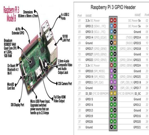
Fig. 2. RPI 3 Model - B with Pin-out diagram
