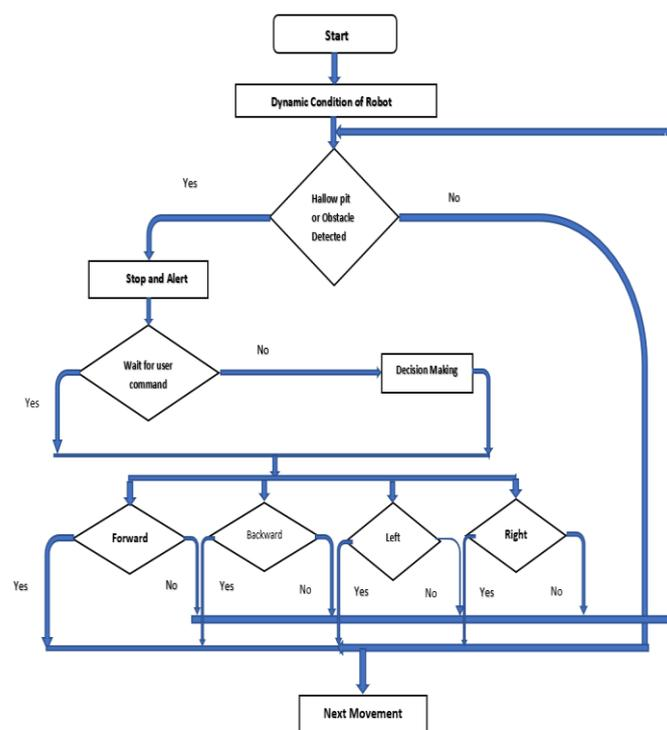
Fig .3. Flow chart for Robot Movement
