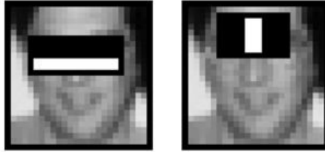
Figure 2(b): HAAR feature used for face in an image
