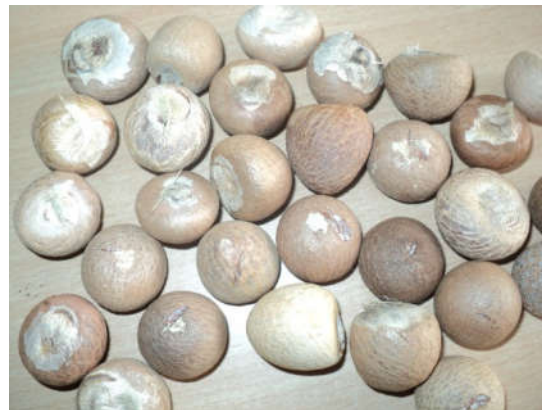
Fig.6 final output of dehusked areca nut
