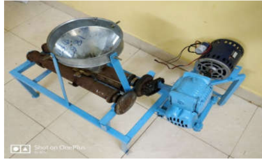
Fig 4: Areca nut dehusking machine
