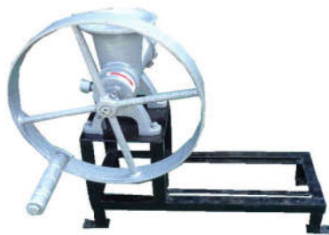
Fig. 2 hand operated peeling machine
